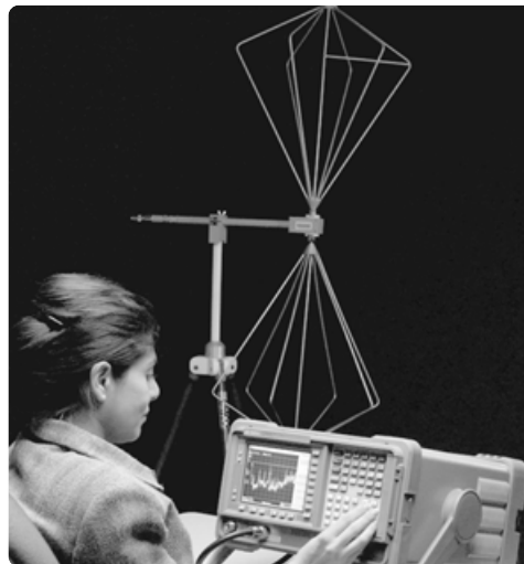
A number of antennas are available with the 84115EM system to test for RF emissions. The E7400 EMC analyzer will also work with other third party antennas.
